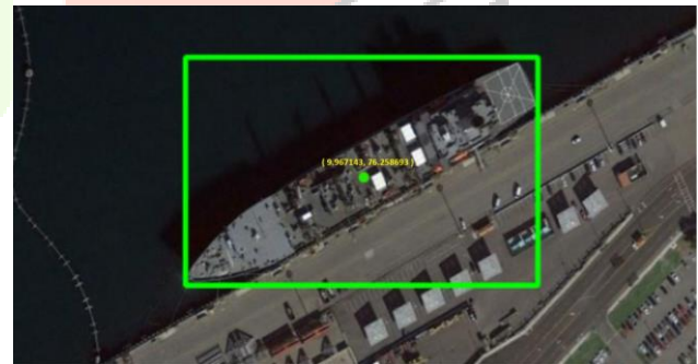
Fig. 15. Detected vessel with bounding box and coordinates
