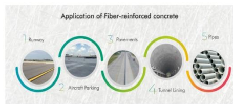
Fig no. 10 Application of fiber-reinforced concrete
