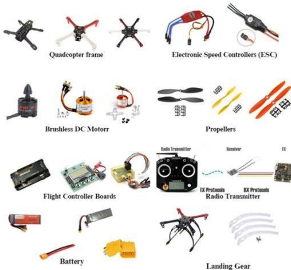
Fig. V.a displays a snippet featuring all the hardware components.
