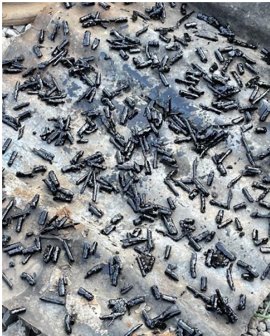
Fig 4: Drying Encapsulated Cigarette butt
