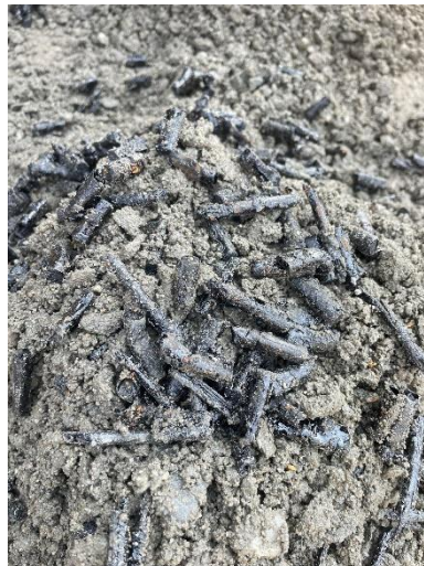
Fig 5: Mixing cigarette butt and concrete
