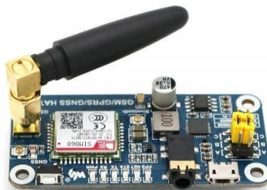
Fig 3.2 GSM(Global System for Mobile Communication) Module
