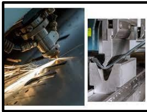
FIG.1.8 Aluminum Sheet - Laser Cutting Technology - Bending Process
