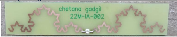
Fig. 4: Koch curve design on 1mm thick FR4
