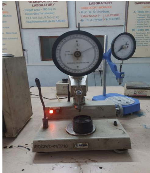
fig.3 – performing penetration test
