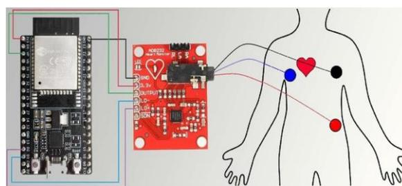
Figure 3: Circuit Diagram
