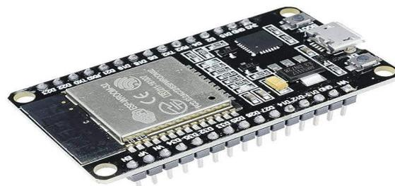
Figure 2: NodeMCU ESP32 Board
