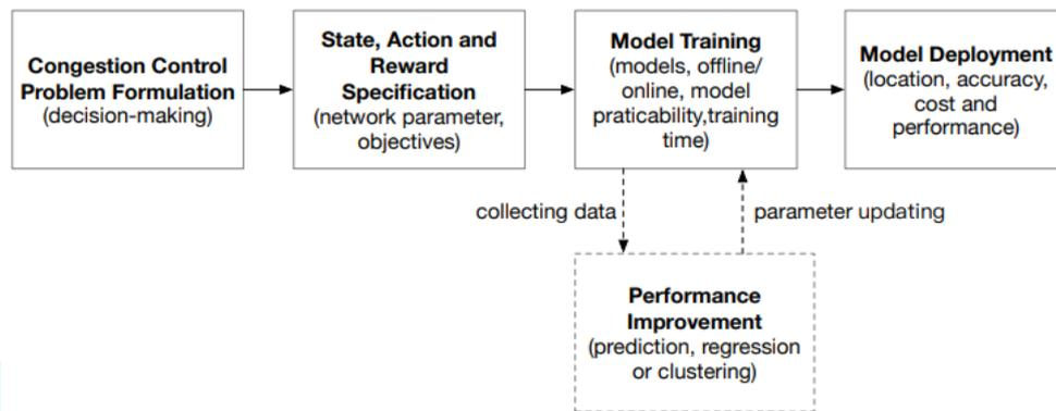
**Figure 1:** Workflow of ML-based congestion control.
