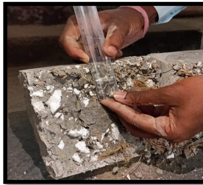
Figure 4 Impermeability Test on floating concrete
