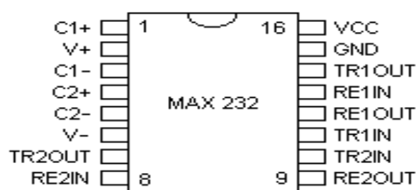
Fig 3. MAX 232 Pin Configuration
