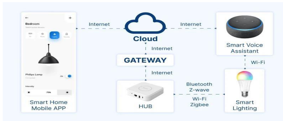
Fig 3: Smart lighting system connected to an IoT gateway
