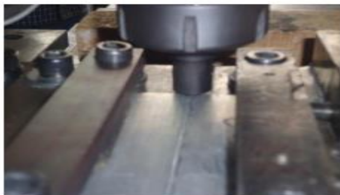
Fig.2.1.Experimental setup for FSW
