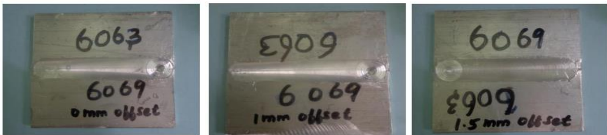
Fig.3.2. Welded Specimens (AA6063- AA6069)
