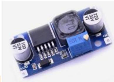
Fig. buck boost converter
