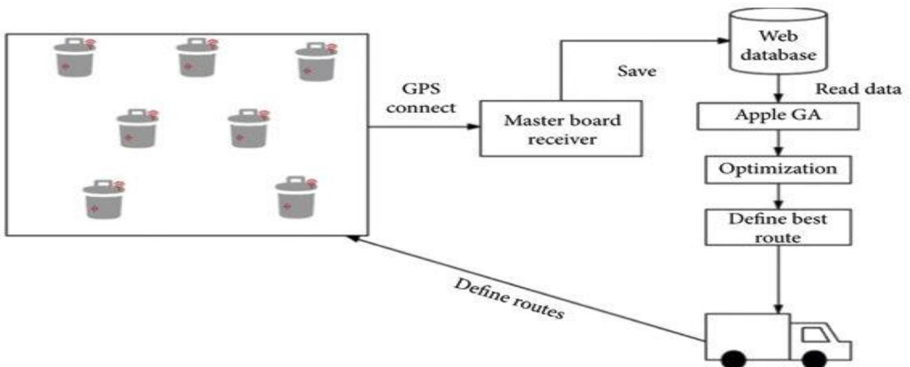
Fig 4. System architecture of SCGCMS
