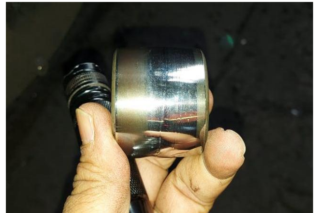
Fig 3(c): collar shows spalling from multiple location; 3(d): Spalled area at collar revealed beach marks
