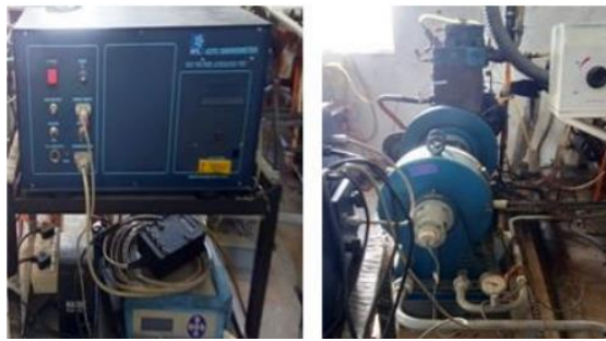
Fig4 :AVL smoke meter and experimental setup
