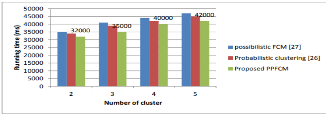
Figure 5: comparative analysis of running time of plants dataset based on number of clusters
