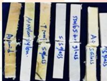
Figure flexural strength specimens of all materials Flexural stresses are determined by the following relations.
