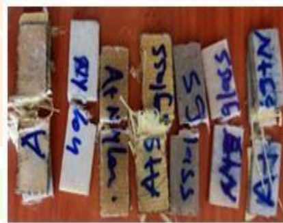
Figure impact strength specimens of all materials The examination Impact strength was calculated by the following relation
