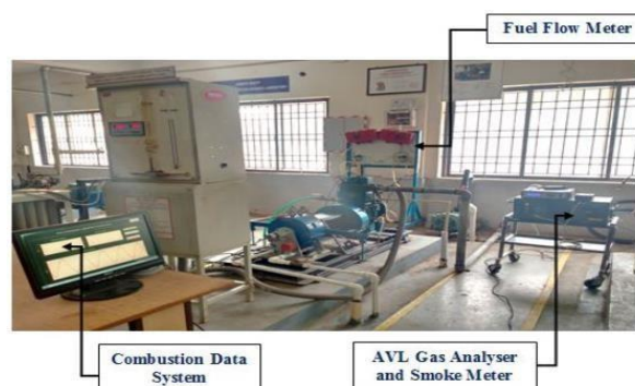
Figure 4 AVL smoke meter and experimental setup
