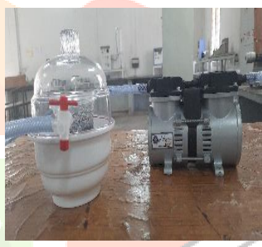
Figure II-3. Operating Vacuum Desiccator with Vacuum Pump
