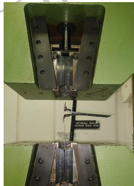
Figure II-6. DCB Test on UTM
