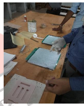
Figure II-4. Hand Lay-Up set up
