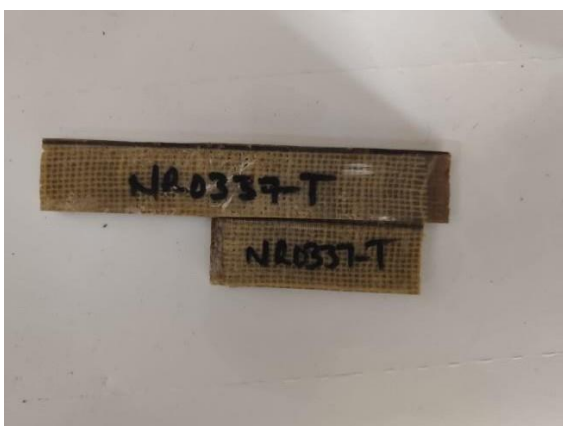
Fig 2a. Specimens as per ASTM for tensile test
