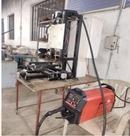
Figure 1: MIG-WAAM process setup
