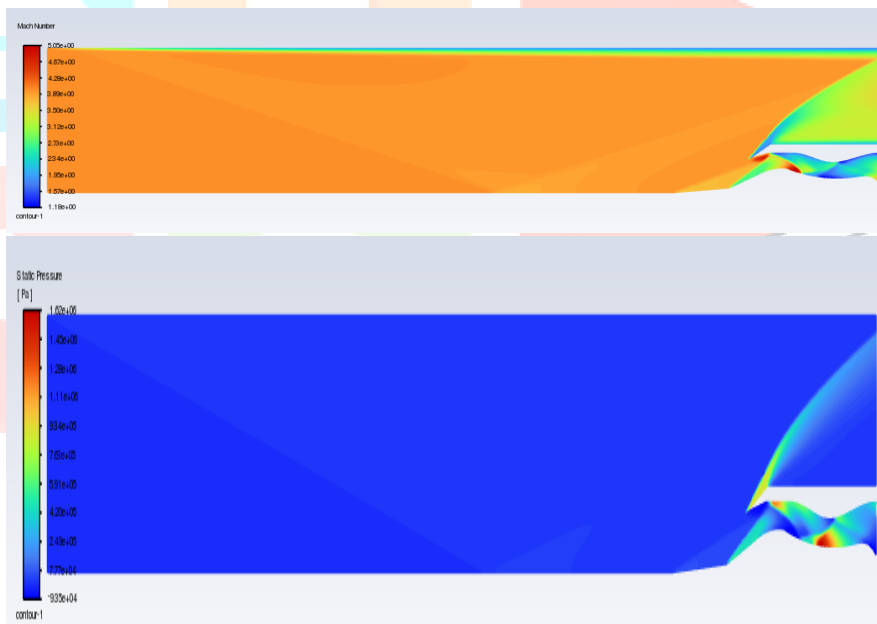
Fig.10: Mach number and pressure distribution in supersonic inlet diffuser for \theta_1=13^\circ , \theta_1=4^\circ , \theta_2=21^\circ
