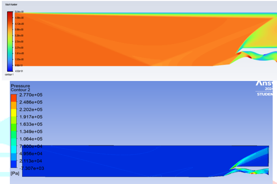
Fig.12: Mach number and pressure distribution in supersonic inlet diffuser for \alpha_1=13^\circ, \alpha_2=4^\circ, \alpha_3=22^\circ
