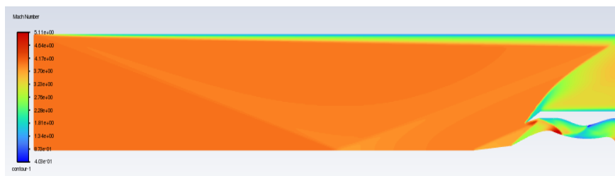
Fig.10: Mach number and pressure distribution in supersonic inlet diffuser for \theta_1=13^\circ , \theta_1=4^\circ , \theta_2=21^\circ
