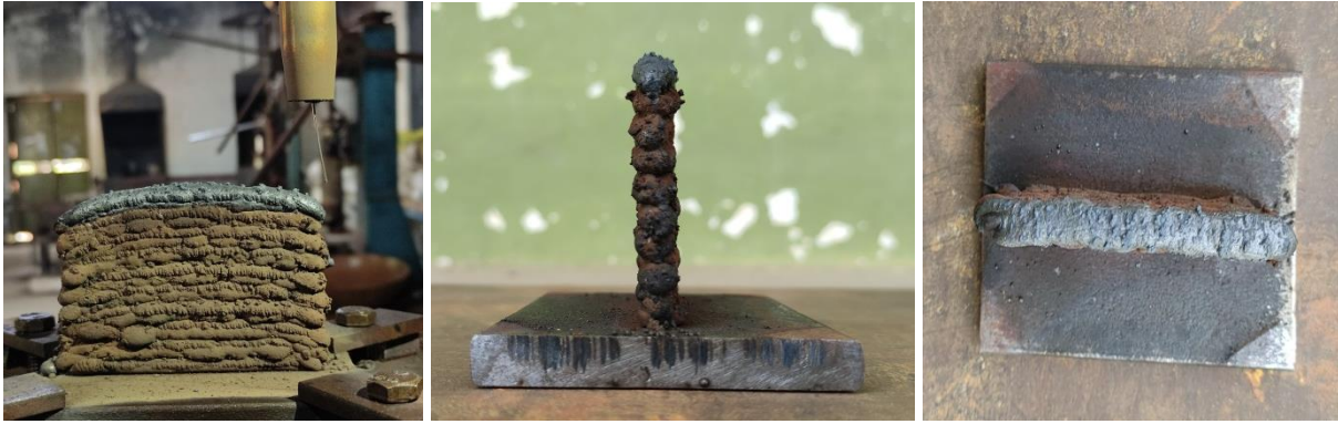
Figure 5. Single wall structure built with optimum set of parameters
