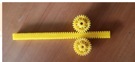
Fig 3: Rack and Pinions
