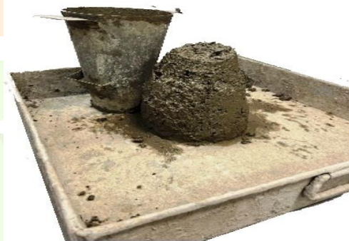
Figure 3 – Slump Test being performed for the concrete mix.
