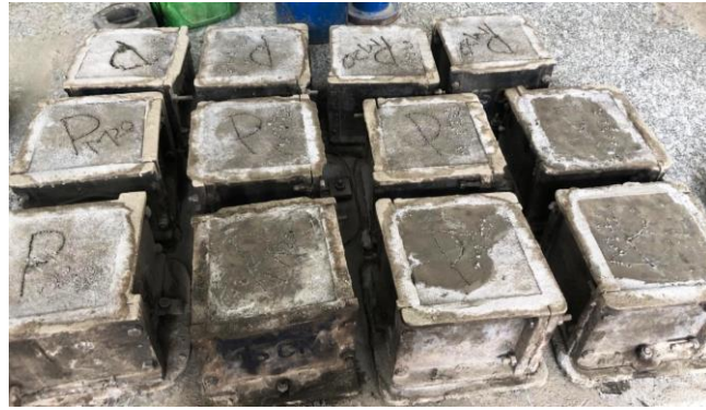
Figure 2 – Sample being prepared for conducting investigation for different concrete mix.
