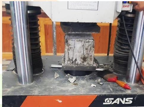
Figure 5 – Compressive Test being performed for the concrete mix.
