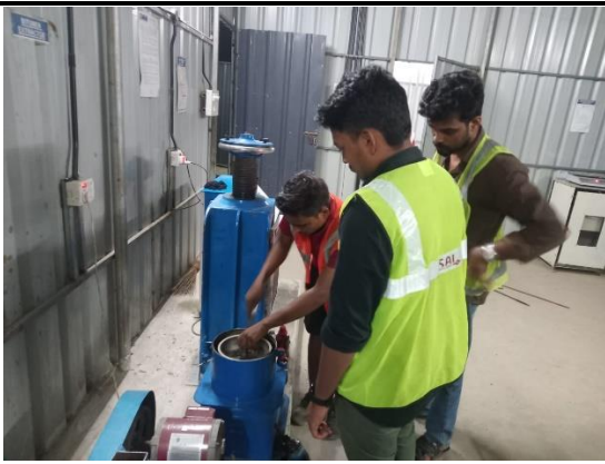
Fig.No.04: Extraction test for bitumen
