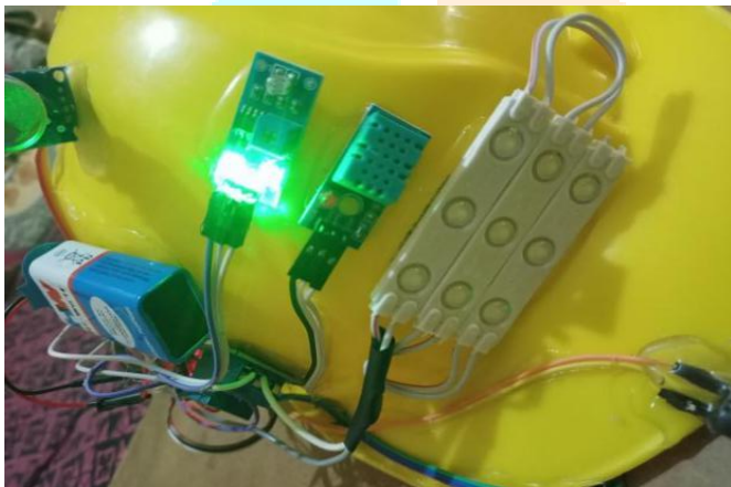
Fig.4: Working of LDR Sensor & ON mode of TORCH
