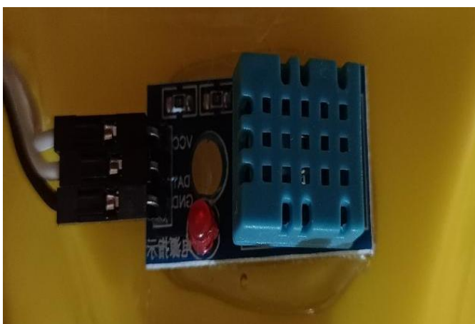
Fig.5: Working of DHT-11 Sensor & Values in Blynk
