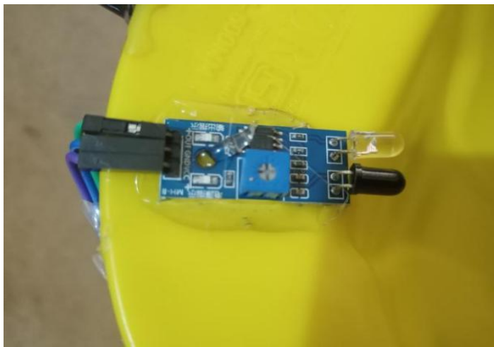
Fig.3: Helmet Removal Alert using IR Sensor
