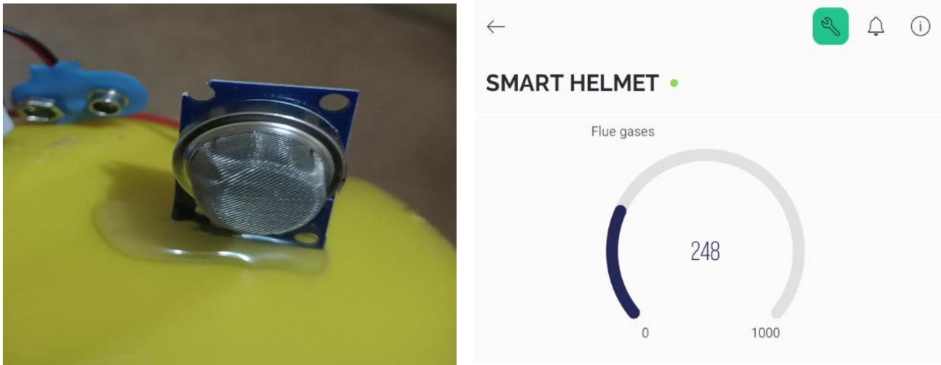
Fig.9: Concentration of Poisonous gases by MQ4 Sensor
