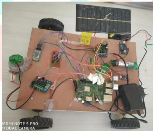
Figure 2: Prototype model of our Robot grass cutter
