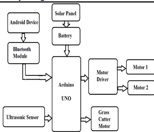
Figure 1: Schematic diagram of the Robotic Solar Grass Cutter
