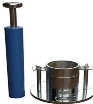
Fig 3.1. Modified Proctor test apparatus
