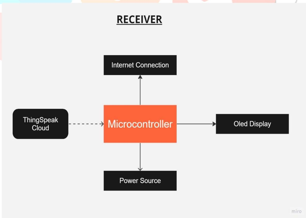
Fig.4.3.1.2 Receiver Block Diagram
