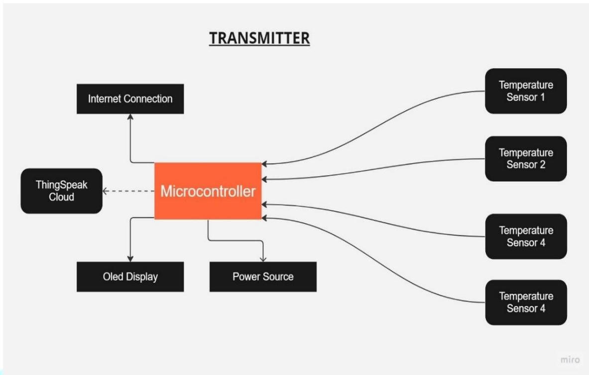
Fig.4.1.1 Transmitter Block Diagram
