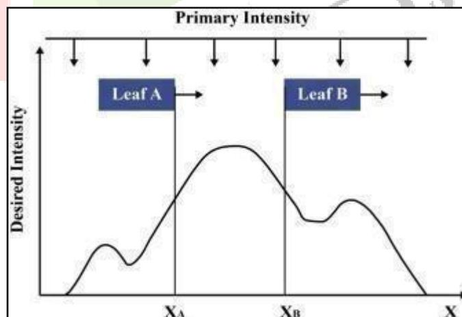
fig. 5: one leaf pair is used to generate a one-dimensional intensity-modulation.
