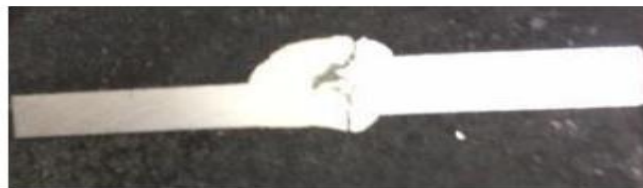
Figure: Sample after etching for micro hardness
