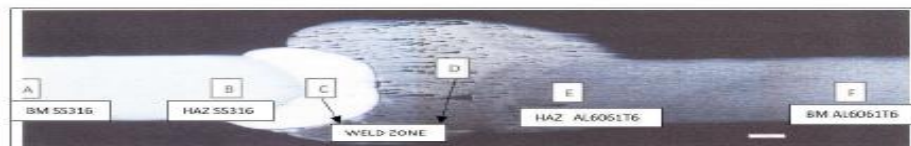
Figure: Sample combination Al 6061-SS316- Microstructure weld zones
