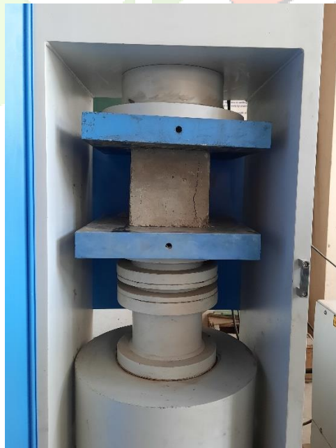
Fig 6: Compressive Strength Test
