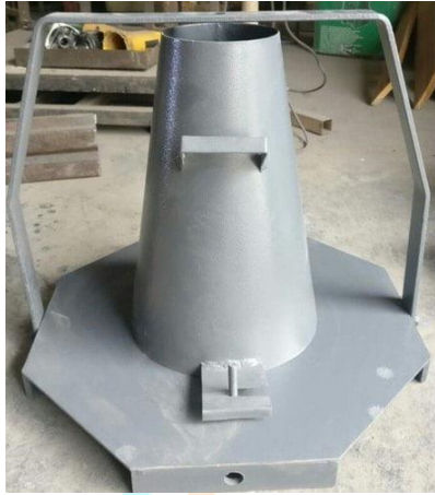
Figure 4.1.1: Slump Apparatus (Dimensions)
