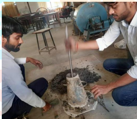
Figure 4.1.3: Tamping Of Concrete Tamping Rod
