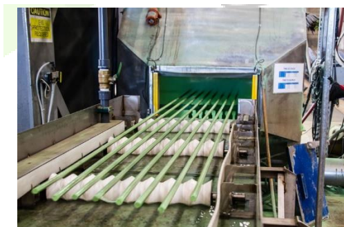
Fig1. Using epoxy as a layer on reinforcement bar
