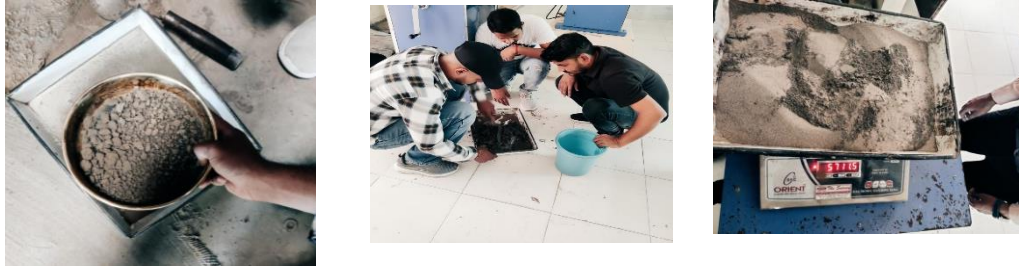
4.REFINING SAND WITH SIEVES
