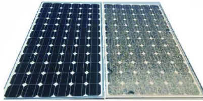
Figure 6: the accumulation of dust is often observed at the periphery of the module frame.
