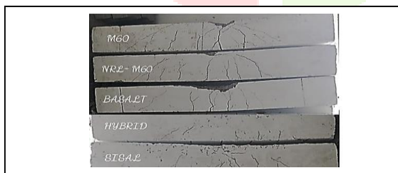
Fig. 3. Crack pattern in beams.
