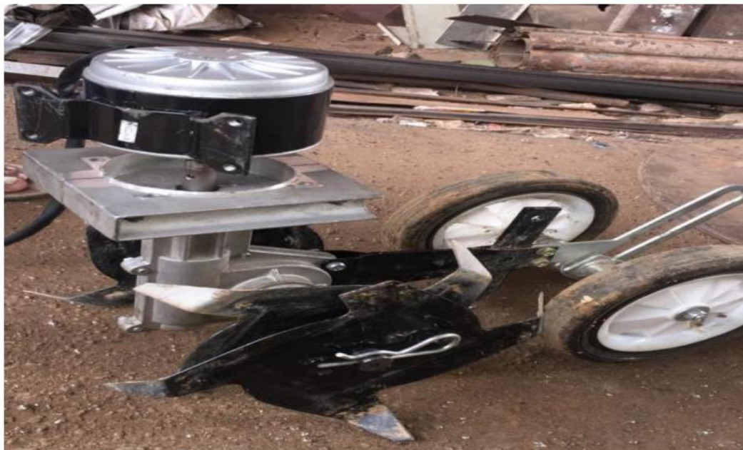
Fig. 4 Assembly of PMDC, gear Shaft with Cultivator
