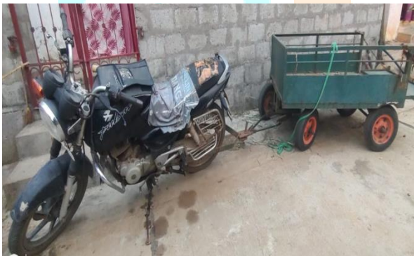
Fig-7: The 4-wheeler trolley is connected to the bike without loading.
