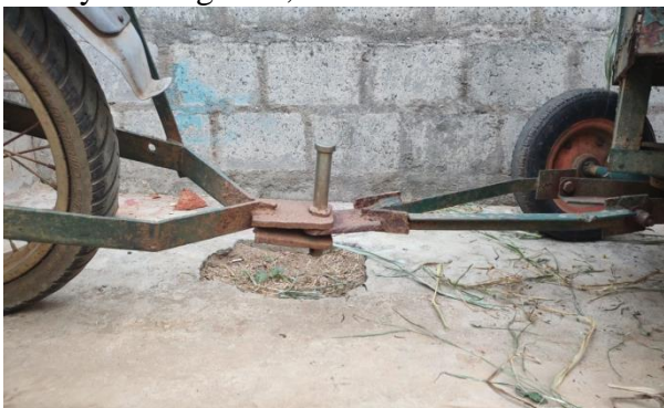
Fig-3: The bike and trolley connecting point.
