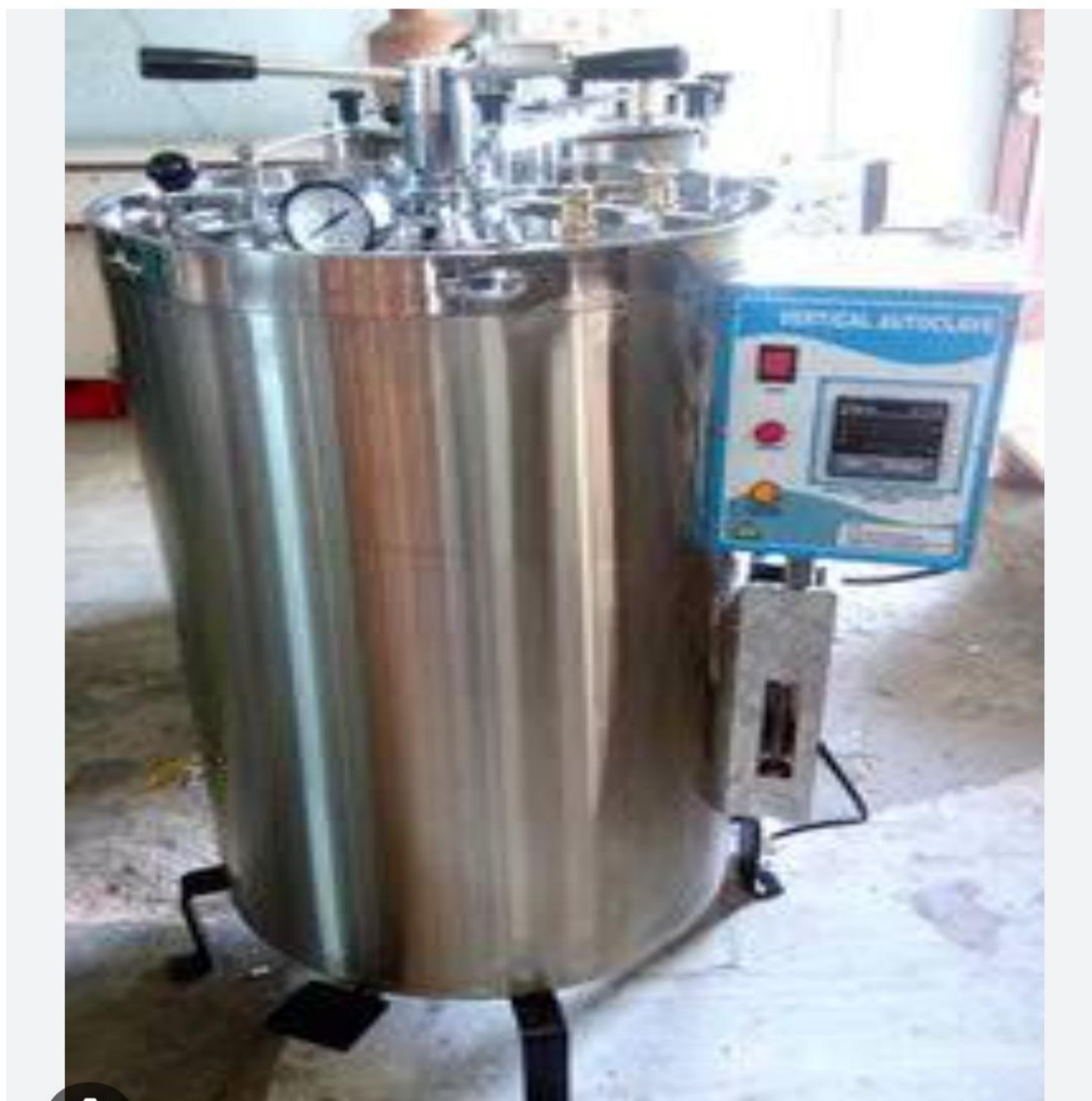
Fig 2 : autoclave operation in biotechnology lab.
