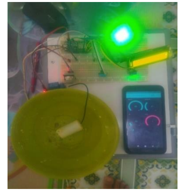
Figure.18. Testing of the water pump
