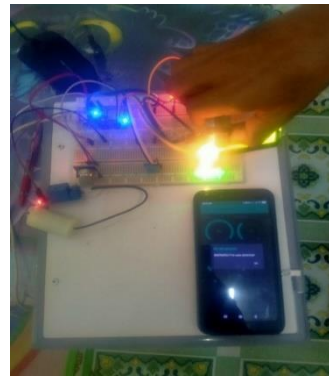
Figure.17. Testing of the humidity sensor
