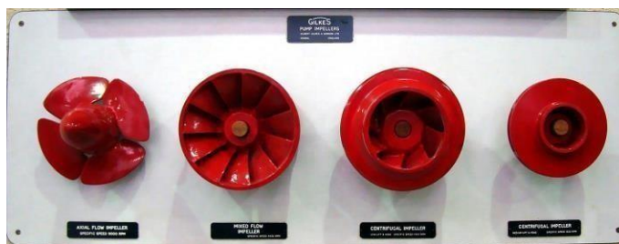
Fig 1. Types of impeller blade
