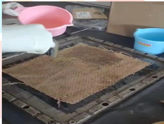
(Applying resin on jute fiber, below the jute consists of carbon fiber)
