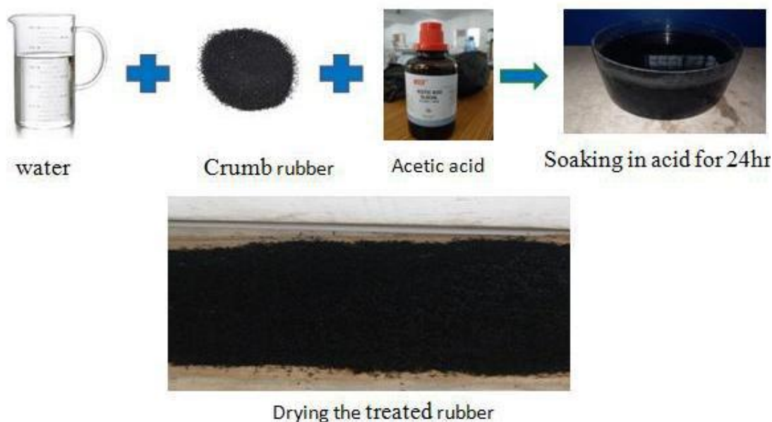
Figure 3.3 Treatment of crumb rubber
