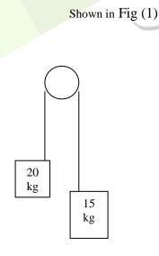
Pulley is mass less and length of strings 20 meters (10 m for each), and 15 kg mass goes below 5 meters.
