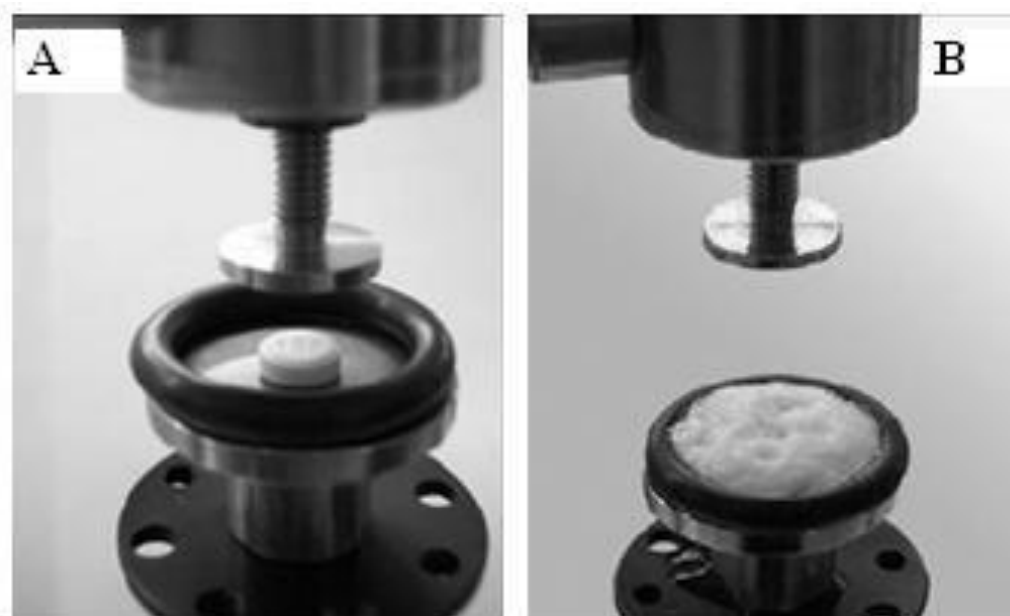
FIG. 8 ELECTROFORCE® APPARATUS FOR DISINTEGRATION TEST
