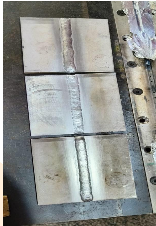
Fig 2.5 TIG welded samples
